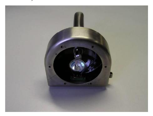
The bulb and reflector assembly (207003, NSN 6240-99-251-7786) is clipped into the bulb holder. Remove the clips then unplug the bulb.
