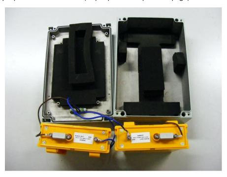
To replace batteries; ensure that all terminal connections are tight (torque 0.6Nm) and check the battery cross volts.
