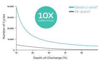
\*Silent Watch Capability: Cycle Life\*\*\* (28.7V charge voltage, "C' rate discharge and +20°C)
